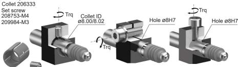
Method 1: Typical Clamping Torque M4 Screw: 0.30/0.35 Nm M5 Screw: 0.35/0.40 Nm Method 2 Clamping Torque dependant on fixturing Method 3: Typical Clamping Torque M4 Screw: 0.25/0.30 Nm M5 Screw: 0.30/0.35 Nm Produces 50 Kg approx. point load
